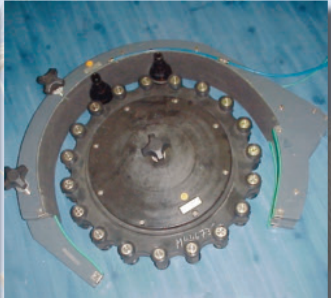
Lifting equipment of labelling machine
